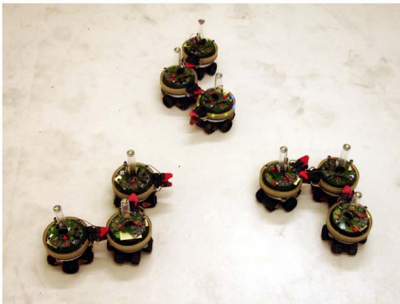
Fig. 13 Communicated-step-replicator script and result. Video 4— Towards Adaptive Morphogenesis in the online supplementary material shows the experiment which produced this result. NB: In this experiment, the pattern on the right is slightly malformed. This was due to the seed robot's connection slot being mis-sensed (due to camera noise) by the first robot to attach
