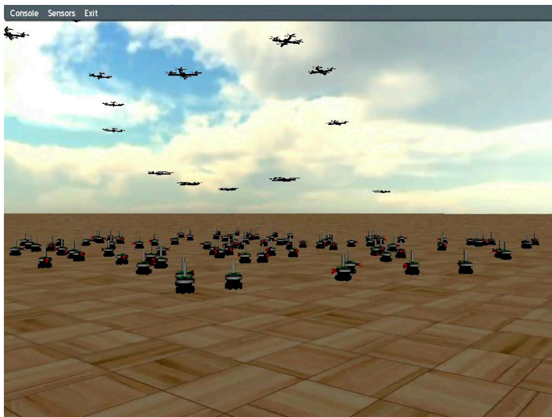
Figure 6.1: An example of a heterogeneous swarm of robots: s-bots navigate on the ground using a differential drive systems, while eye-bots are quad-rotor flying robots with long-range sensing capabilities.
