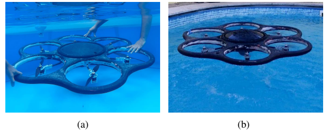
Fig. 8. Preliminary validation in a swimming pool. (a) The UAV fully submerged. (b) The UAV hovering above the water surface.
