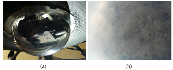
Fig. 6. Video acquisition system. (a) Gimbal placed inside the UAV structure with a plastic dome. (b) Underwater images retrieved using the UAV's monocular camera.
