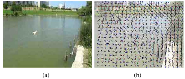
Fig. 2. Trackers on a typical video sequence. (a) Frame on which trackers were deployed. (b) Trajectories performed by the trackers across n frames. Red dots represent trackers’ initial positions, whereas the blue dots represent trackers’ final positions. Off water non-linear trajectories are a result of severe camera rotation. Nevertheless, they are not as complex as the trajectories of the trackers deployed on water nor as unpredictable. See for instance that the trajectories of neighbour trackers on water are much more different from each other than the trajectories of neighbour trackers off water.
